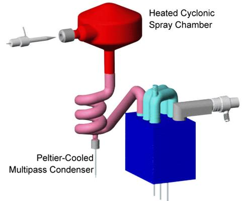
Custom temperature settings for heater and cooler. Patented flow path design ensures rapid wash-in / washout.
